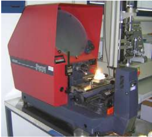
Figure 7 The profile projector used for the measurements.
