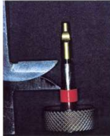
Figure 13. The analog is connected to the fixture mount (Winsix Ltd.), with the red band guiding placement depth.
