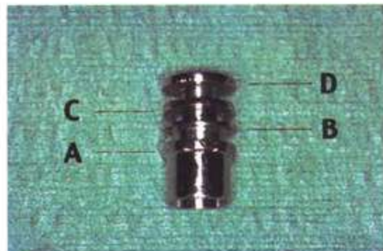
Figure 10. Additional sleeves (B, C, and D) are attached to sleeve A. The sleeves can be removed 1 at a time.
