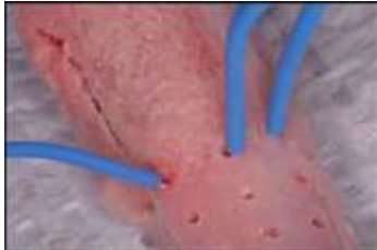
Fig. 1. Three canals for thermocouples at different depths (2, 5, and 9 mm) were drilled on the external surface of each specimen. The implant sites were done on the upper surface of the specimen.
