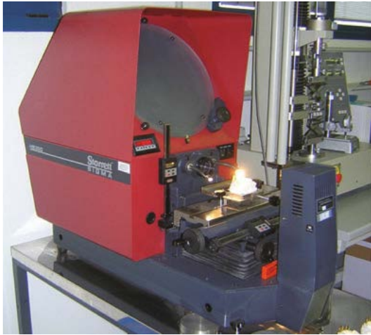
Figure 7 The profile projector used for the measurements.
