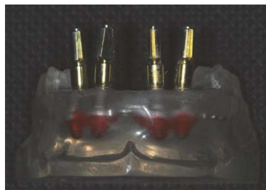
Figure 5 The master model CTR2: the longitudinal axes of the anterior implants had 5° convergence toward the midline whereas the longitudinal axes of the posterior implants had 5° divergence away from the midline.
